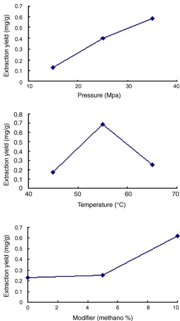
Fig. 2. Effects of temperature, pressure and modifier concentration on extraction yield.
