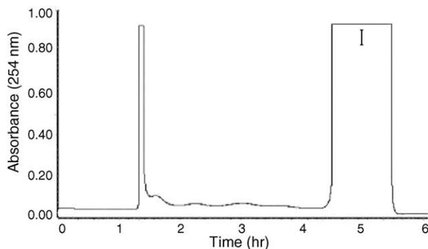
Fig. 4. Chromatogram of the crude extract II by preparative HSCCC. Solvent system: *n*-hexane–ethyl acetate–methanol–water (1:1.2:1.2:1, v/v/v/v); stationary phase: upper phase; mobile phase: lower phase; flow rate: 2.0 ml/min; revolution speed: 800 rpm; sample size: 400 mg; retention of stationary phase: 63%; sample loop: 20 ml; detection wavelength: 254 nm.
