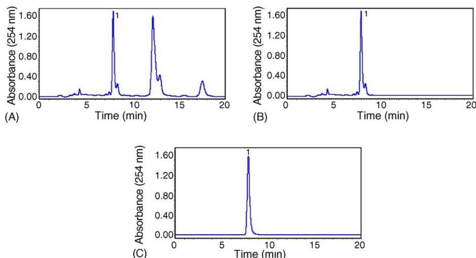
Fig. 3. HPLC chromatogram of the samples. (A) Crude extract I before silica gel step; (B) crude extract II after silica gel step; (C) fraction (155 mg) obtained by HSCCC; column: reversed-phase Lichrospher C<sub>18</sub> (6.0 mm × 150 mm i.d. 5 μm); mobile phase: CH<sub>3</sub>CN–H<sub>2</sub>O (80:20, v/v); flow rate: 1.0 ml/min; UV wavelength: 254 nm; peak 1: aurentiamide acetate.
