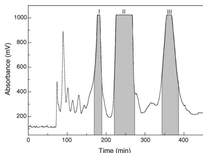
Fig. 3. HSCCC chromatogram of crude extract from *Epimedium koreamum* Nakai. Two-phase solvent system: chloroform–methanol–water (4:3.5:2, v/v); mobile phase: the lower phase; flow-rate: 2.0 ml min<sup>-1</sup>; revolution speed: 900 rpm; detection wavelength: 254 nm; sample size: 200 mg of crude sample dissolved in 4 ml of the upper phase; separation temperature: 25 °C; retention percentage of the stationary phase: 50%.
