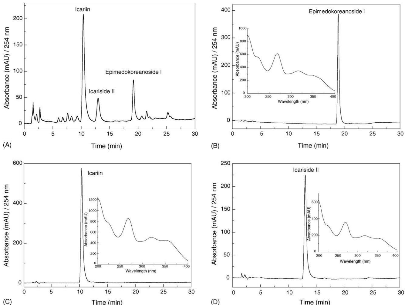
Fig. 2. HPLC chromatogram of crude extract from *Epimedium koreamum* Nakai and HSCCC peak fractions. Conditions: column: reversed phase YWG C<sub>18</sub> column (200 mm × 4.6 mm i.d., 10 µm); mobile phase: acetonitrile and water in gradient mode (acetonitrile: 0–12 min, 28%; 12–20 min, 28–35%; 20–30 min, 35%); flow-rate: 1.0 ml min<sup>-1</sup>; detection wavelength: 254 nm. (A) Crude extract from *Epimedium koreamum* Nakai; (B–D) HSCCC peak fractions I–III in Fig. 3.
