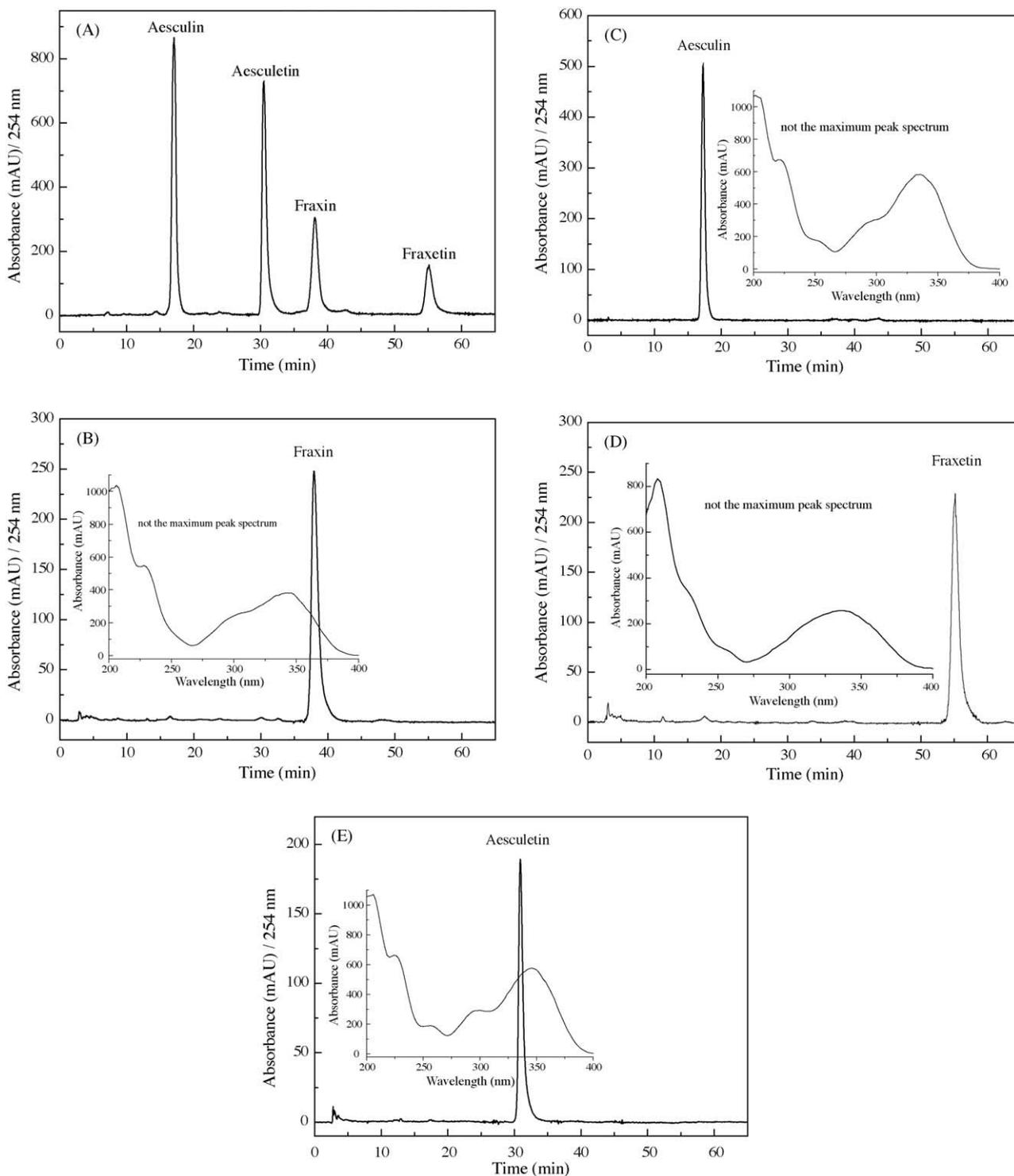
Fig. 2. HPLC chromatogram of crude extract from *Cortex fraxinus* and HSCCC peak fractions. Conditions: column: SPHERIGEL ODS-C<sub>18</sub> column (250 mm × 4.6 mm i.d., 5 μm); mobile phase: methanol–0.1% phosphoric acid (16:84, v/v); flow-rate: 1.0 ml min<sup>-1</sup>; detection wavelength: 254 nm. crude extract from *Cortex fraxinus*; (B)–(E) HSCCC peak fraction I–IV in Fig. 3.
