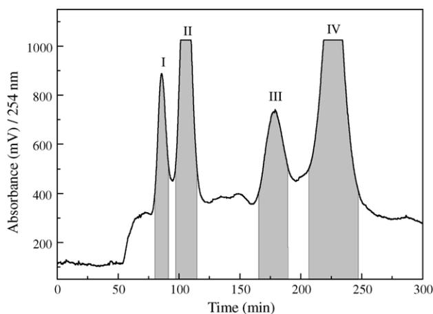
Fig. 3. HSCCC chromatogram of crude extract from *Cortex fraxinus*. Two-phase solvent system: *n*-butanol–methanol–0.5% acetic acid (5:1.5:5); mobile phase: the lower phase; flow-rate: 1.5 ml min<sup>-1</sup>; revolution speed: 900 rpm; detection wavelength: 254 nm; sample size: 150 mg of crude sample dissolved in 5 ml of the upper phase; separation temperature: 25 °C; retention percentage of the stationary phase: 30%.
